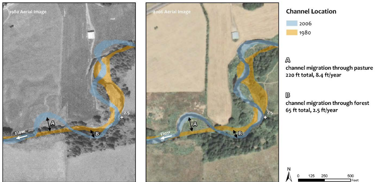
Figure 28. Differences in erosion rates of pastured versus forested land along the North Fork Newaukum River at RM 2.5 between 1980 and 2006. A shows rapid erosion into a pasture. B shows slower erosion into forest area. Rapid erosion into pastures is evident in the upper right.
